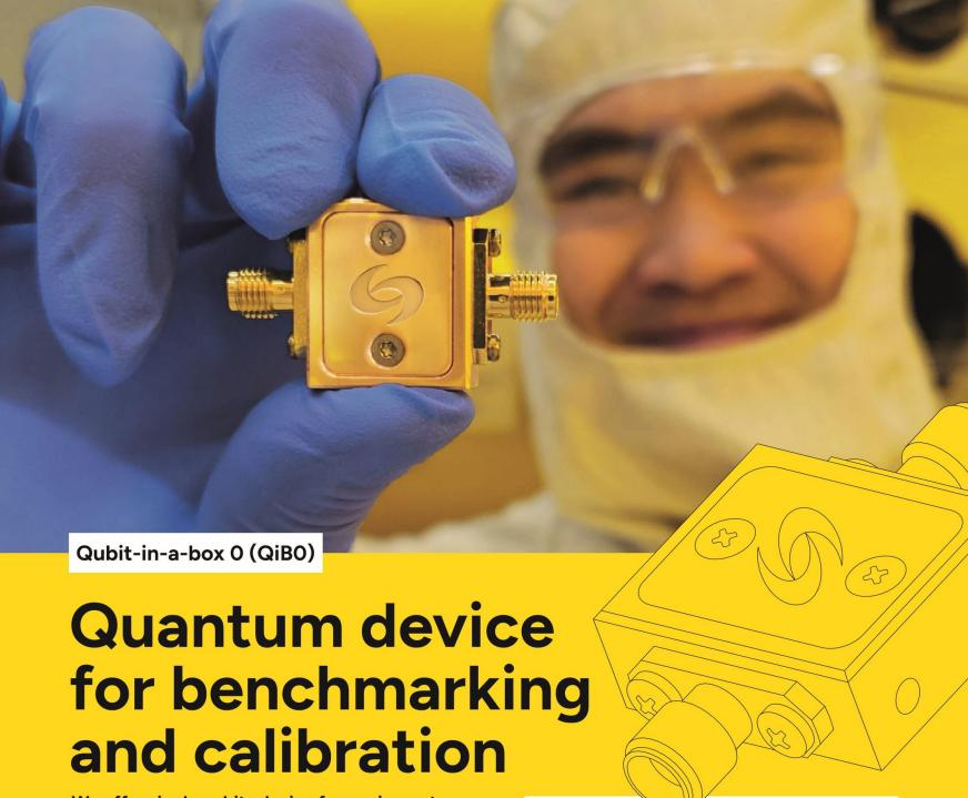
We offer single qubits device for equipment and cryostat testing with world class Qubit performance. The device can be used to benchmark your quantum measurement system or demonstrate simple quantum processes such as decoherence and dephasing.
